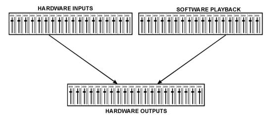
TotalMix can be used in the above view (View Options **2** Row). However, the default is a vertical alignment in three rows as known from an Inline desk, so that the row *Software Playback* equals the *Tape Return* of a real mixing desk:
