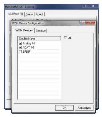
The screenshot to the left shows the multi-channel WDM devices available with the Multiface after selecting 'Multi-Channel' in the WDM Devices listbox and hitting WDM Configure. In this example the devices Analog 1 to 8 and ADAT 1 to 8 are active.
