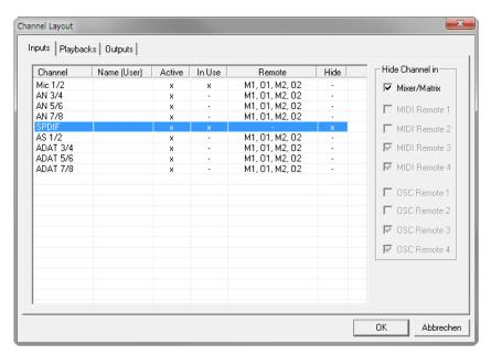
Rows Inputs, Playbacks and Outputs are set up individually by the tabs at the top. *Active* indicates currently available channels. At higher sample rates many ADAT channels are no longer active. *In Use* shows which channels are currently used in the mixing process.
