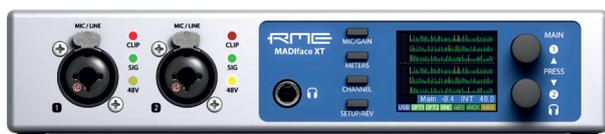
The front of the MADiface XT has 2 XLR/TRS line and microphone inputs, a stereo line/headphone output, two rotary encoders with push functionality, four menu keys, a graphical colour display, and six status LEDs.
