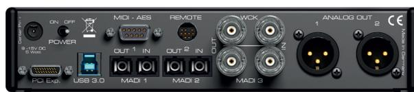
The rear panel has two balanced analog outputs, word clock I/O, MADi coaxial I/O, two MADi optical I/O, USB 3 port (compatible to USB 2), PCI Express connector, MIDI/AES I/O D-sub for breakout cable, the power socket and a power switch.
