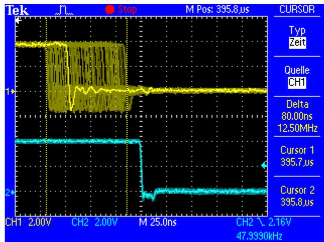
The other input sources of the MADiface XT, word clock and AES, gain a lot from SteadyClock as well. In fact, extracting a low jitter clock from LTC is not possible without a Steady-Clock similar technique at all!
