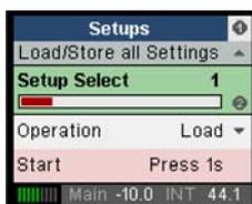
The MADiface XT can store and load its current state in 6 different memory slots, called Setups. With this, the MADiface XT can be used stand-alone after setting it up accordingly, replacing lots of dedicated devices (see chapter 24).
